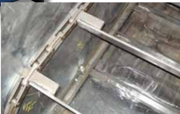
Heavy duty construction of internal tracks provides a positive vacuum seal.
