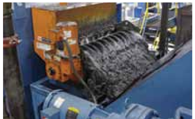
Cast iron can be scalped using magnetic rolls improving the efficiency of the filter and reducing media consumption.
