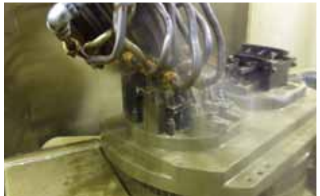
Precision grinding using high pressure cutting fluids
